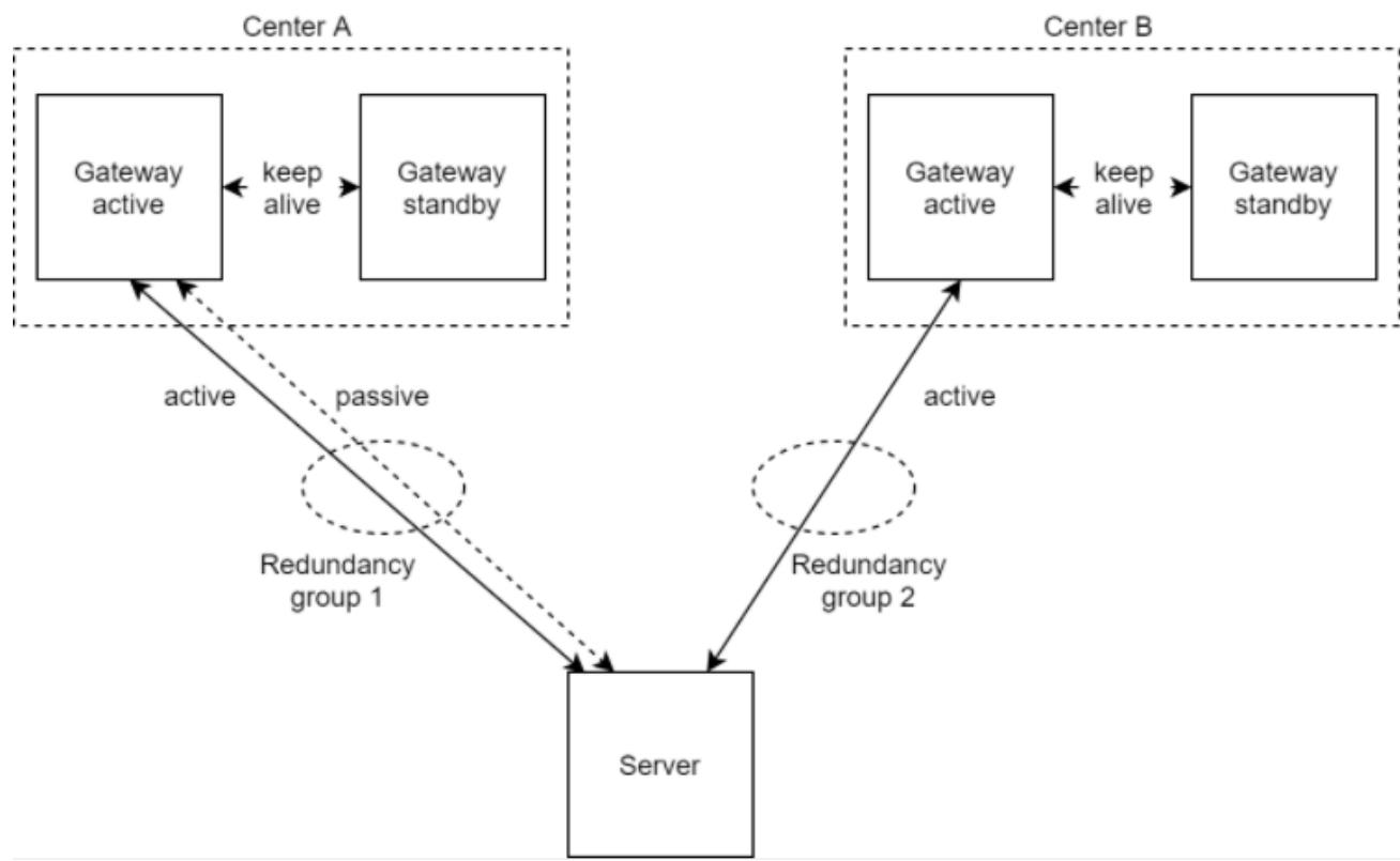
In this example, 2 control centers, center A and B, are establishing communication with the server.
